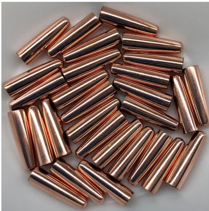
**Fig. 1:** O-free and P-doped copper “bullet” electrodes.
