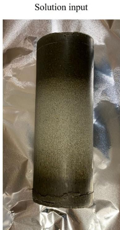
**FIGURE 3** Saturation profile of a bentonite sample extracted from a pressure vessel. Bentonite was compacted to  $1600 \text{ kg/m}^3$  for an experimental duration of 1 month. [Color figure can be viewed at [wileyonlinelibrary.com](https://onlinelibrary.wiley.com)]
